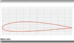
mum thickness of the airfoil as a percentage of the chord. A NACA 0015 airfoil is symmetrical, with the 00 occupying the first two digits indicating it has no camber.
