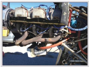
The author's uncowled engine, a Lycoming IO-540. The air filter assembly is the white object below it. The fuel servo is mounted above the air filter assembly's aft portion. That orange hose is the fuel line, contained in fire-sleeving material.
